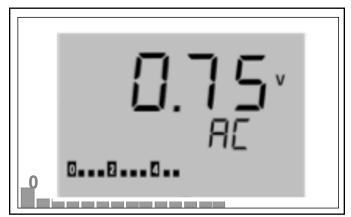
Figure 9. AC voltage display
