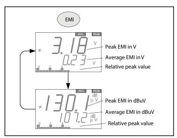
Figure 12. EMI Measurement screen
