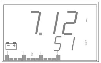
Figure 5. Battery voltage and percentage.
