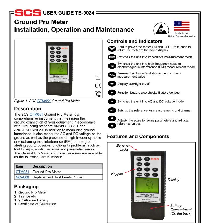
Figure 2. Ground Pro Meter features and components
