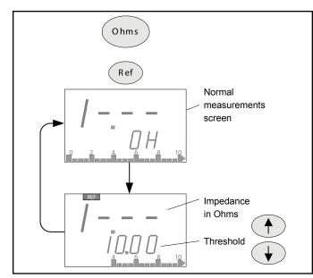
Figure 11. Impedance measurements screen
