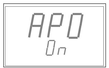
Figure 4. Automatic Power Off (APO) display
