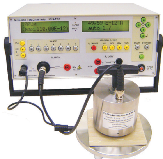
Volume resistance measurement with FBE 4 and earth plate GP 14 (optional) and Milli-TO 3
