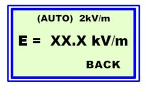
In the 1st. line it shows the selected Measure Mode => AUTO and the actual Range => 2kV/m. In the 2nd line it shows by E-Feld Measurement  $\rightarrow$  E = (actual value) kV/m
